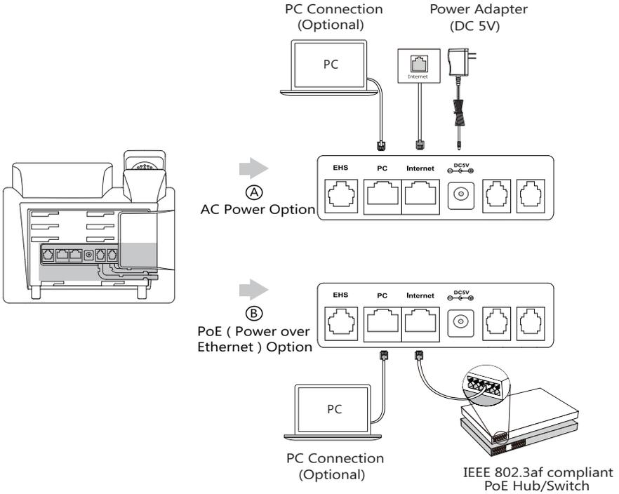
**Note:** The IP phone should be used with Yealink original power adapter (5V/600mA) only. The use of the third-party power adapter may cause the damage to the phone. If you are connecting a PC to your phone, we recommend that you use the Ethernet cable provided by Yealink. If inline power (PoE) is provided, you do not need to connect the power adapter. Make sure the hub/switch is PoE-compliant.
